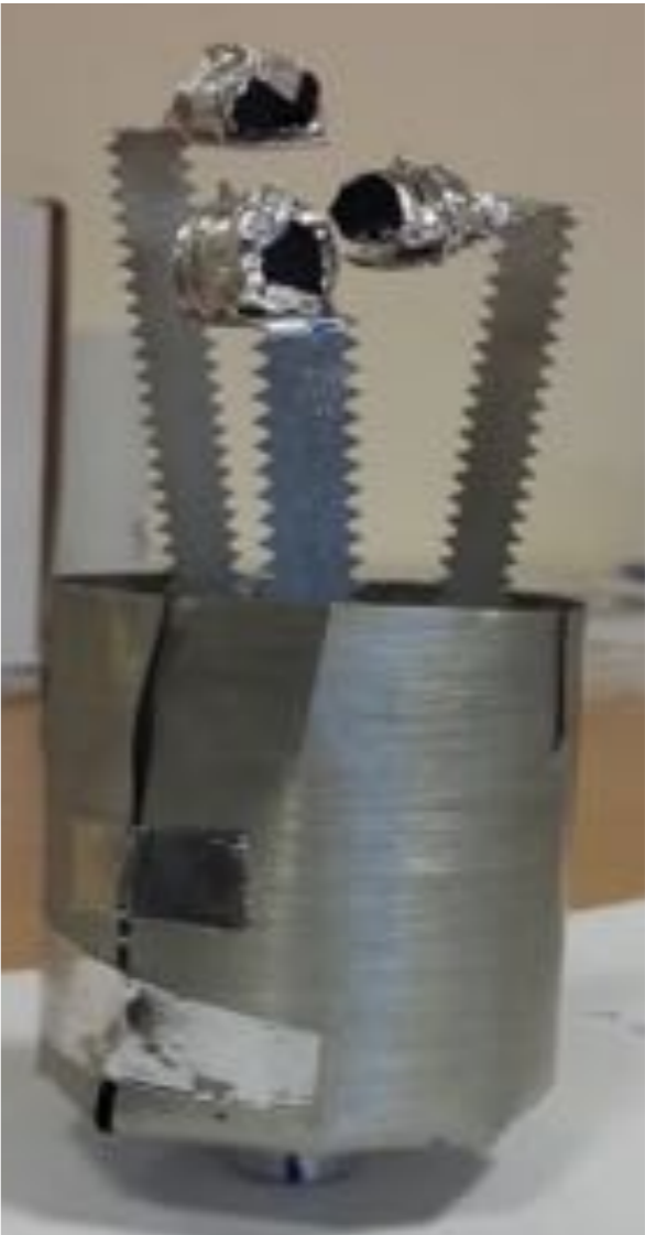
Three co-aligned single crystals for INS experiment
